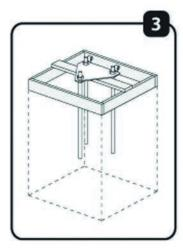
Put the prepared "Foot set" in a hole so that the longest part of the threaded rods would be in the hole, but the mast foot bottom plate with a free thread up would be above the hole level. Mast foot bottom plate above the hole must be leveled.
