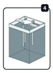
With a pre-prepared concrete mortar mix fill the hole and level the mast foot bottom plate for the second time.
