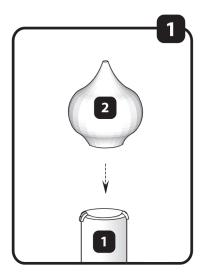
Connect nozzle (2) with rotating part built in ( agpole (1), bolting or ffxing it on (depending on nozzle type).
