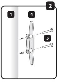
With the help of screws (5) bolt handle (4) to secure rope to flagpole (1) in its intended place - bottom of the mast.
